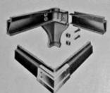
are made up of a heavy strip of Wellsville Polished Steel stamped into shape and backed with a reinforcing strip electrically welded to it. The corners of the cabinet base and the legs of the leg base are cast iron, nickel plated and bolted to the steel side strips. Both of these bases are of a pleasing design and take up no more floor space than the range without base.
